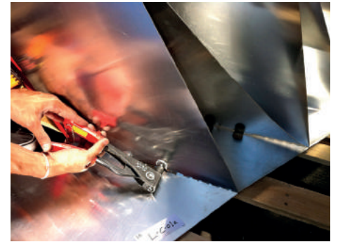
Fig. 10: The aluminium was folded and riveted into corrugated layers.
