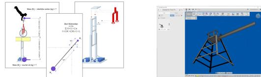
The design phase consisted of calculations for torque, 3D CAD models for the towers, and a spreadsheet for building a new unicycle wheel. Design reviews were held to re-evaluate the design choices as the design matured.
